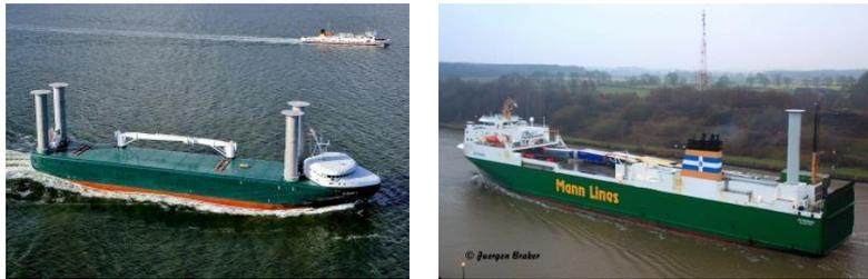
Figure 1 E-Ship 1 (Enercon Wind Company) and Estraden *Ro-Ro* cargo (Norsepower Company)
